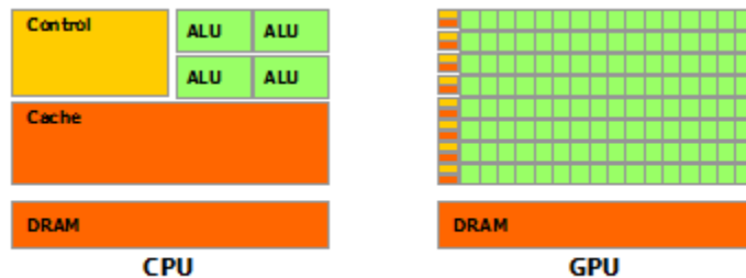
Figure 2.1: CPU/GPU Architectural Differences [24]
