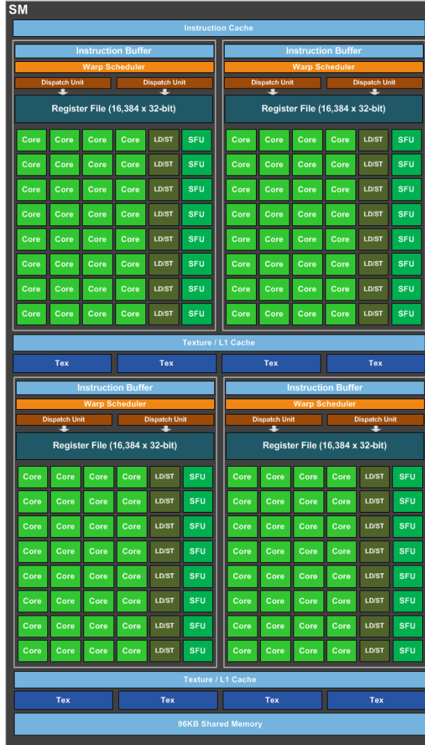
Figure 4.1: GeForce GTX 1080 Streaming Multiprocessor [25]
